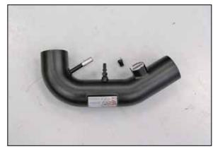
19. On vehicles equipped with an EVAP vent line, install the provided quick disconnect fitting into the K&N® intake tube. On vehicles not equipped with the EVAP vent line, install the provided 1/4npt plug into the K&N® intake tube.
