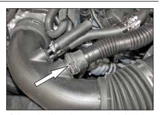
5. Release the clamp that secures the pulse hose to the intake tube and then remove the pulse hose from the vehicle.
