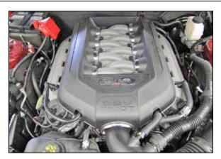
3. Lift up the engine cover to dislodge it from the mounts and then remove it from the vehicle.
