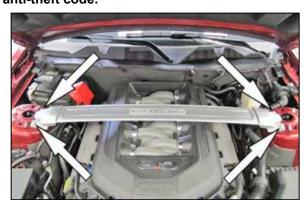
2. On vehicles equipped with a strut tower brace, remove the four nuts that secure the brace and then remove the brace from the vehicle.
