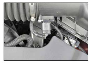
7. Disconnect the mass air sensor electrical connection
