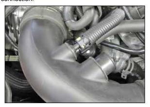
8. Disconnect the crank case vent hose from the intake tube.
