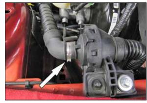
4. Cut the clamp that secures the engine pulse hose to the drum and disconnect the hose from the drum.
