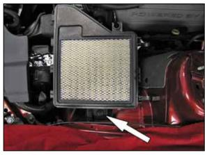
11. Remove the bolt that secures the lower air box to the inner fender and then remove the lower air box from the vehicle.
