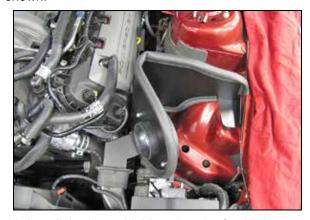
16. Install the heat shield so that the fresh air scoop enters into the factory duct and align the mounting hole with the rubber mounted stud, then secure with the provided hardware.
