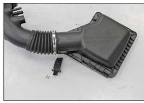
20. Remove the two screws securing the mass air sensor into the upper air box and then remove the mass air sensor from the air box.
