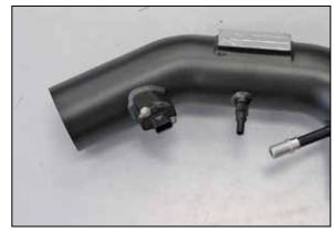
21. Install the mass air sensor into the  $K\&N^{\mbox{\scriptsize @}}$  intake tube and secure with the provided hardware.
