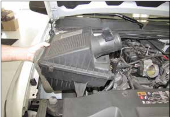
8. Pull firmly upward to release the air cleaner assembly from the mounting tray grommets. Then remove the assembly as shown. NOTE: K&N recommends that customers do not discard factory air intake.
