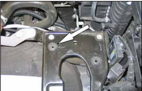
13. Remove the air box mounting grommet shown from the air box mounting plate.
