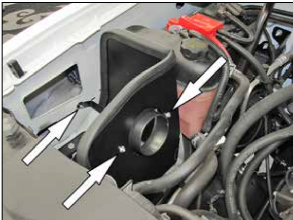
19. Secure the mounting bracket to the inner fender with the hardware provided. Then Install the filter adapter onto the heat shield and secure with the provided hardware.
