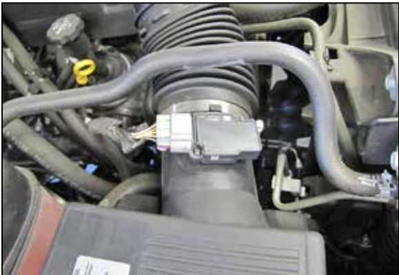
2. Disconnect the mass air electrical connection.
