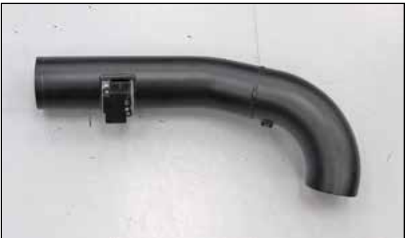
10. Install the mass air sensor into the K&N® intake tube and secure with the provided hardware.
