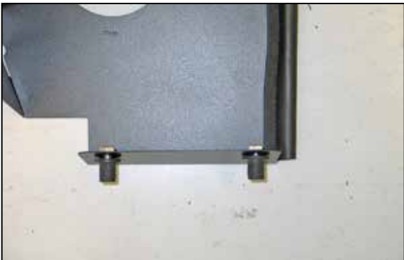
17. Install the reaming 5/16" inserted nut into the heat shield as shown.
