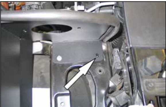
15. Set the heat shield assembly into position with the inserted nut installed into the air box mounting grommet location. Mark the heat shield mounting location to be drilled.
