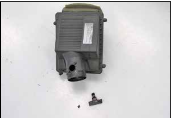
9. Remove the two screws securing the mass air sensor to the air box and then remove the mass air sensor from the air box as shown.
