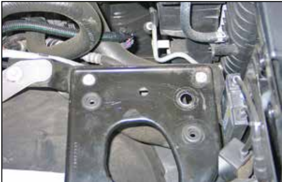
16. Remove the heat shield assembly and drill a 5/8" hole at the marked location.
