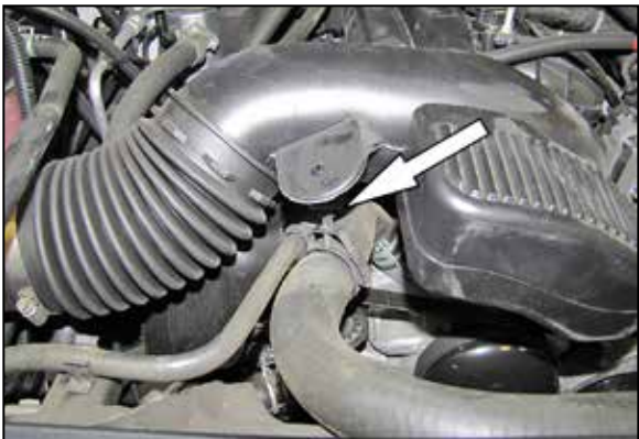
4. Unhook the radiator hose mount from the intake tube.
