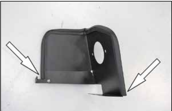
12. Install the provided edge trim onto the heat shield as shown. Note: Some trimming will be necessary.
