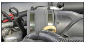
15. Install the provided hump hose (08617) onto the turbo inlet and secure with the provided hose clamp.
