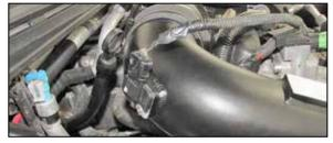
18. Connect the mass air sensor electrical connection.
