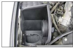
11. Install the heat shield assembly onto the filter mounting plate and secure with factory bolts from step #5.
