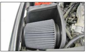
12. Install the K&N<sup>®</sup> air filter onto the filter adapter and secure with the provided hose clamp.
