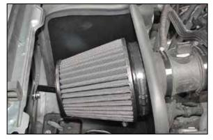
26. Install the K&N<sup>®</sup> filter as shown and secure with the provided hose clamp.
