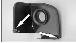
11. Install the provided edge trim onto the heat shield as shown. **NOTE: some trimming of the edge trim mat be**
