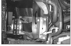
13. On vehicles not equipped with the front air box mounting grommet and hole, install the heat shield assembly as shown. Then use a marker to mark the mounting plate through the heat shield mounting hole.
