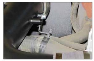
24. Install the upper radiator hose mount onto the mounting bracket installed onto the K&N<sup>®</sup> intake tube.
