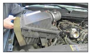
7. Pull firmly upwards to release the air cleaner assembly from the mounting tray grommets, and then remove the assembly as shown. **NOTE: K&N Engineering, Inc., recommends that customers do not discard factory air intake.**
