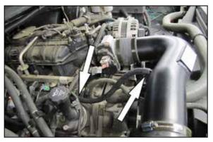
25. Install the provided crank case vent hose onto the valve cover and then onto the K&N $^{\odot}$  intake tube as shown.
