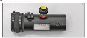
29. Install the provided silicone hump hose (08418) onto the  $K\&N^{\otimes}$  intake tube.
