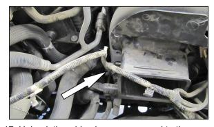
17. Unhook the wiring harness secured to the core support through the fresh air intake duct.
