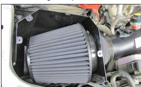
34. Feed the K&N® air filter top first into its location then rotate it back and install onto the filter adapter. Secure the air filter with the provided hose clamp.
