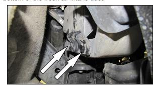
15. Remove the two clips shown that retain the bottom of the fresh air intake duct.
