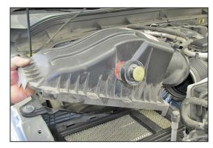
5. Remove the upper air box housing from the vehicle.
