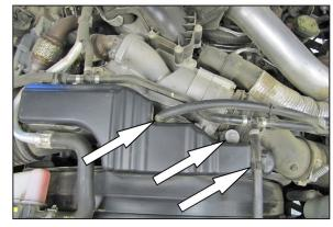
6. Unhook the coolant hoses from the intake plenum and remove the bolt securing the plenum to the engine fan shroud.
