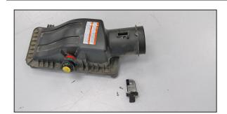
25. Remove the two screws securing the mass air sensor into the factory air box and then remove the sensor from the air box.
