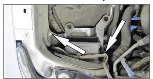
11. Remove the two bolts which secure the air box mounting bracket to the core support and inner fender.
