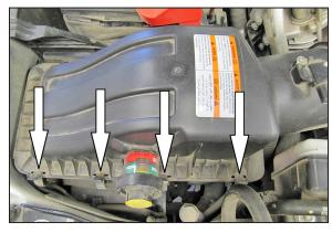
4. Release the four upper air box retaining clips.
