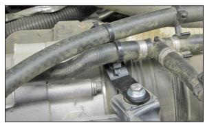
33. Install the coolant hose bracket onto the fan shroud and then secure the coolant hoses with the provided mounting tie wraps as shown.
