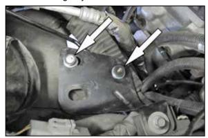
10. Install the two provided rubber mounted studs onto the air box mounting tray as shown.
