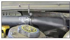
4. Unhook the warm air inlet tube from the firewall as shown.
