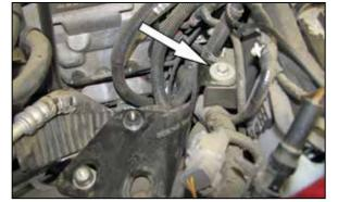
11. Remove the battery tray mounting bolt shown. **NOTE: This bolt will be reused.**
