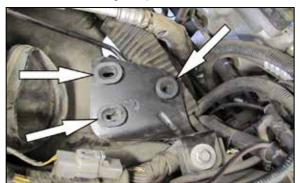
9. Remove the three mounting grommets from the air box mounting tray.
