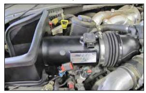
15. Install the K&N® intake tube into the factory inlet hose and align with the mounting bracket. Secure the tube with the factory hose clamp and hardware provided.
