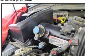
16. Install the factory filter minder grommet and filter minder as shown.
