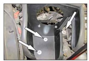
12. Install the heat shield assembly into position so that it rests onto the rubber mounted studs. Secure the heat shield onto the rubber mounted studs with the provided hardware and to the battery tray with the bolt removed in the previous step.
