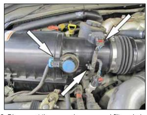
2. Disconnect the mass air sensor and filter minder electrical connections and unhook the wiring harness clip from the air box.
