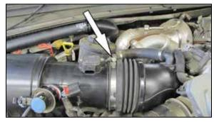
3. Loosen the hose clamp securing the inlet hose to the air box.
