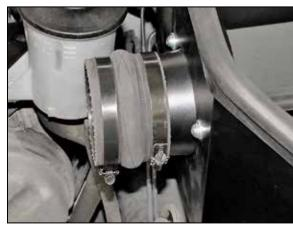
17. Install the provided hump hose (084057) onto the filter adapter and secure with the provided hose clamp.
