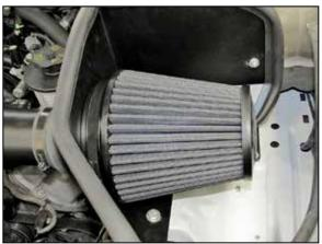
23. Install the  $K\&N^{\otimes}$  air filter onto the filter adapter and secure with the provided hose clamp.
