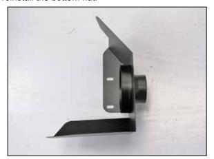
11. Install the filter adapter into the heat shield as shown and secure with the provided hardware.
