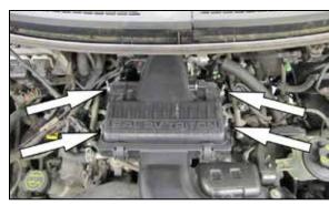
6. Remove the four bolts securing the air filter housing to the intake manifold.
