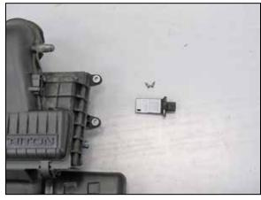
18. Remove the two screws securing the mass air sensor into the stock air filter housing and then remove the sensor from the vehicle.
