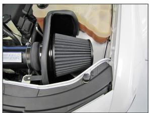
24. Install the K&N<sup>®</sup> air filter and secure with the provided hose clamp.
