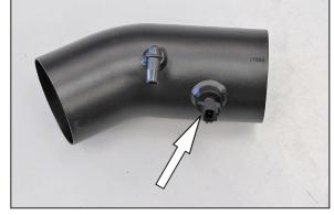
17. Install the inlet air temperature sensor into the  $K\&N^{\circledast}$  intake tube as shown.
