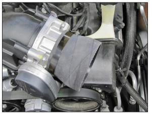
14. Install the silicone step hose (08050) onto the throttle body and secure with the provided hose clamp.
