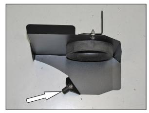
10. Install the provided inserted nut onto the heat shield as shown and secure with the provided hardware.
