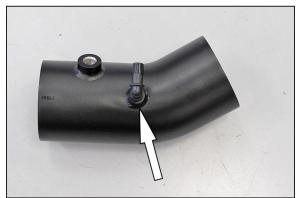
15. Install the provided 90° vent fitting into the K&N<sup>®</sup> intake tube as shown.
