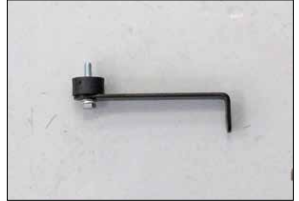
18. Install the provided rubber mounted stud onto the heat shield bracket (083164) as shown.
