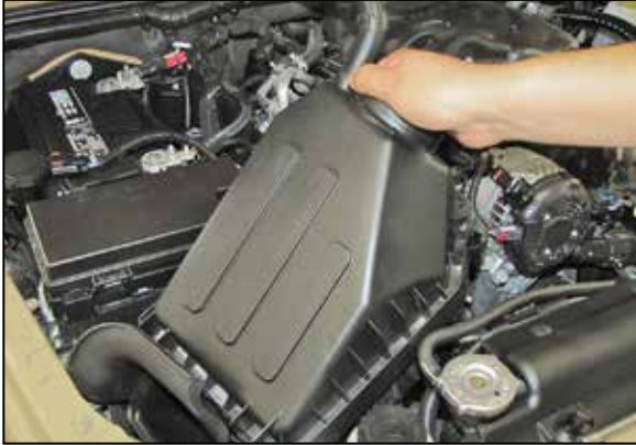
8. Lift up and remove the air filter housing from the vehicle. NOTE: K&N Engineering, Inc., recommends that customers do not discard factory air intake.
