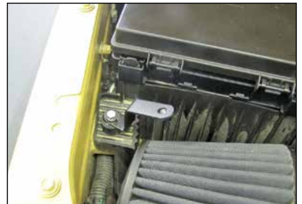
21. Install the provided bracket (083163) onto the rubber mounted stud using the provided hardware.
