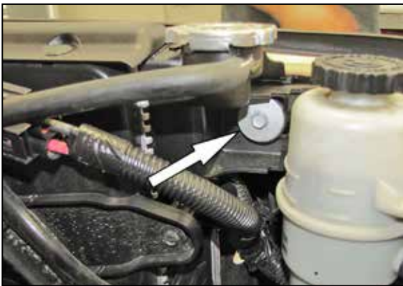
10. Remove the bolt show that secures the radiator to the core support. NOTE: This bolt will be reused in a later step.
