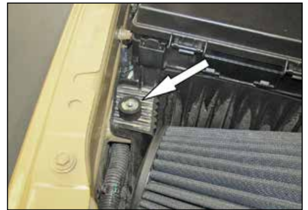
20. Install the rubber mounted stud into the into the air box mounting plate bolt location as shown.
