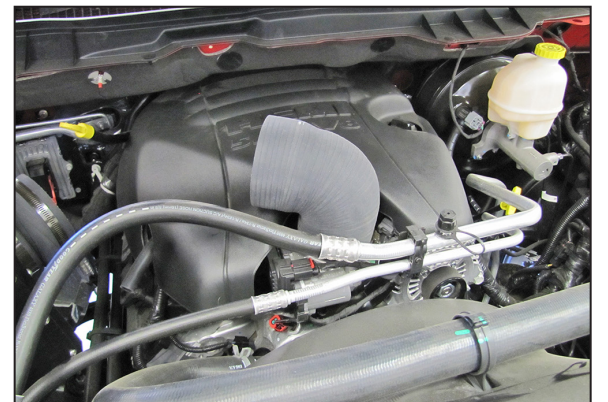
22. Install the provided silicone hose (08498) onto the throttle body and secure with the provided hose clamp. NOTE: Do not completely tighten at this time.
