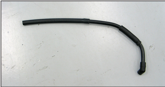
9. Install the provided silicone crank case vent hose onto the cut hose as shown.
