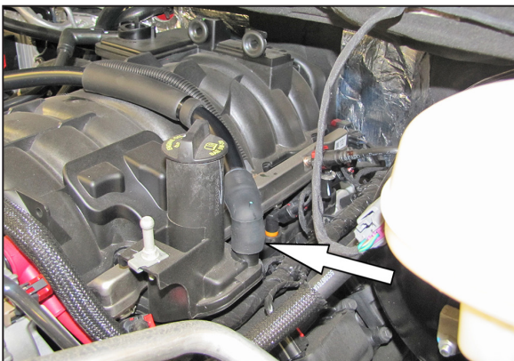
10. Reinstall the crank case vent hose assembly onto the valve cover.
