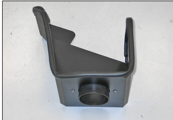
15. Install the provided filter adapter into the K&N® heat shield and secure with the provided hardware.
