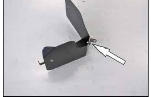
11. Install the tube mounting bracket (070712) onto the heat shield as shown using the provided hardware and spacer.
