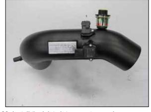
23. Install the inlet air temperature and mass air sensors into the K&N<sup>®</sup> intake tube using the provided hardware.
