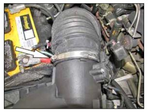
4. Loosen the hose clamp which secures the intake hose to the upper air box housing.
