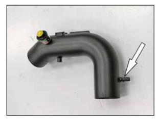
22. Install the 5/8 barb, 1/4npt crank case vent fitting provided into the K&N<sup>®</sup> intake tube as shown.
