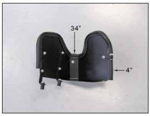
15. Install the edge trim onto the heat shield as shown.
