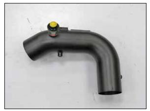
21. On vehicles equipped with a filter minder, install the factory grommet and filter minder into the K&N<sup>®</sup> intake tube as shown.
