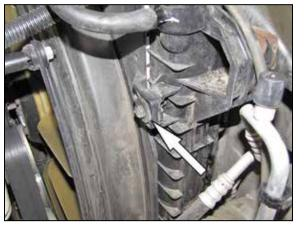
16. Remove the fan shroud bolt shown.
