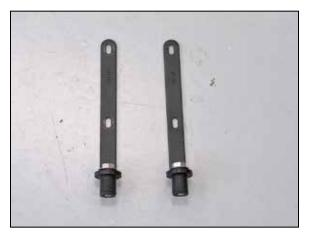
12. Install the 3/8 insert nuts onto the heat shield mounting brackets (07159) using the provided hardware.
