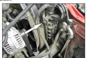
13. Remove the factory fan shroud retaining bolt shown.
