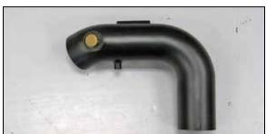
19. On vehicles equipped with a filter minder, drill a 5/8"id hole 6" from end of tube and then install the factory filter minder and grommet.
