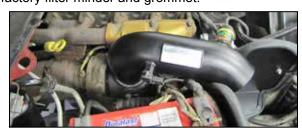
20. Install the K&N® intake tube into the silicone hose installed during step #16 and align with the mounting bracket installed onto the heat shield. Adjust the hose and tube for proper fit and then secure the hose and tube with the provided hardware.
