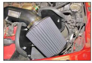
21. Install the K&N® air filter onto the K&N® intake tube.
