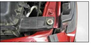
5. Remove the air box mounting bolt shown.
