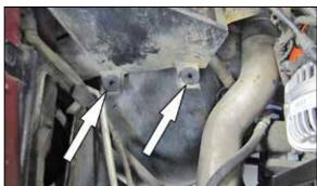
14. Install the two provided inserted nuts into the air box mounting grommet locations.
