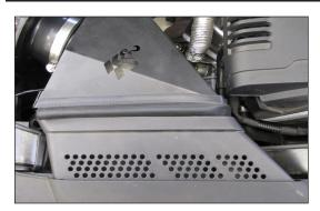
25. Reinstall the factory fresh air scoop onto the core support as shown using the factory hardware.
