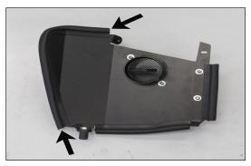
16. Install the 17" section of edge trim onto the heat shield as shown.
