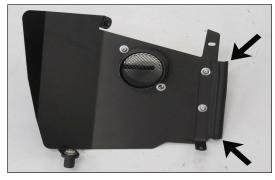
14. Install the 7" section of edge trim onto the heat shield as shown.
