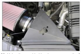
23. Using the provided hardware, secure the fresh air scoop to the heat shield as shown.
