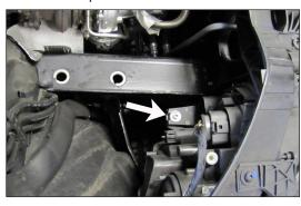
18. Remove the headlamp mounting bolt shown.
