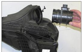
11. Remove the two screws securing the mass air sensor to the air box and then remove the mass air sensor from the air box.
