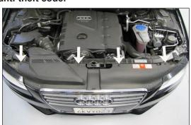
2. Remove the four screws which secure the front core support cover.
