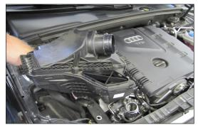
8. Pull up the air box and remove it from the vehicle.
