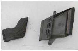
24. Separate the fresh air bellows from the fresh air scoop as shown.
