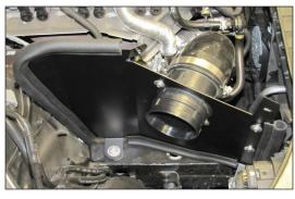
20. Set the heat shield assembly into position on the inner fender while installing the silicone hose onto the turbo inlet. Secure the heat shield with the provided hardware and secure the silicone hose with the provided hose clamps.
