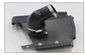
19. Install the silicone hose (08490) onto the mass air sensor as shown and secure with the provided hose clamp.
