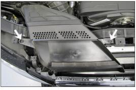
4. Remove the two screws which secure the fresh air scoop to the core support.
