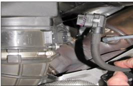
6. Disconnect the mass air sensor electrical connection.
