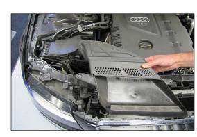
5. Unsnap the fresh air scoop from the air box and then remove the scoop from the vehicle.
