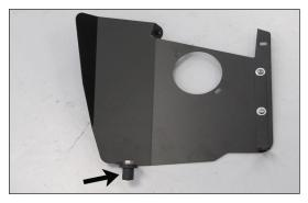
10. Install the inserted nut onto the heat shield using the provided hardware as shown.
