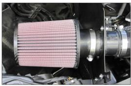
21. Install the K&N® air filter onto mass air sensor and secure with the provided hose clamp.
