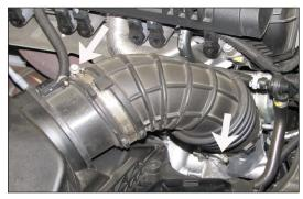
7. Loosen the two hose clamps which secure the stock intake tube to the turbo inlet and factory air box, then remove the intake tube from the vehicle.
