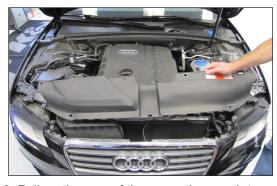
3. Pull up the rear of the cover then push towards the rear to unhook it from the grill. Then remove the cover from the vehicle.
