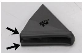
17. Install the 19" section of edge trim onto the fresh air scoop as shown.
