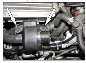
6. Remove the two bolts securing the sound drum to the engine and then remove the sound drum and hose from the vehicle.
