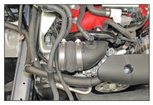
14. Install the provided coupling hose (08185) onto the turbo inlet and secure with the provided hose clamp.
