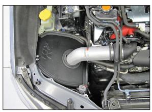
16. Install the intake assembly onto the frame and inner fender then install the intake tube into the coupling hose. Adjust the tube and heat shield for best fit and secure with the provided hose clamp and heathware.
