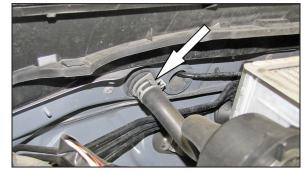
5. Release the spring clamp securing the sound tube to the fitting in the firewall.
