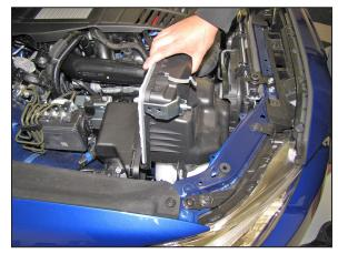
4. Release the two clips and then remove the front half of the air filter housing and air filter from the vehicle.
