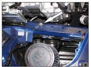
14. Install the provided rubber mounted stud into the air filter housing mounting location on the frame rail.
