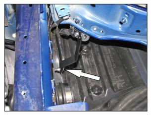
11. Install the tube mounting bracket (064327) into the factory intake tube mounting location using the provided hardware. One section will be 30" long, one section will be 15-1/2" long and the final section will be 3" long.
