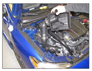
7. Separate the intake tube from the turbo inlet tube and remove the assembly from the vehicle. **NOTE: The hose separation may be difficult due** to the location and tight clearance. **NOTE: K&N Engineering, Inc., recommends that** customers do not discard factory air intake.
