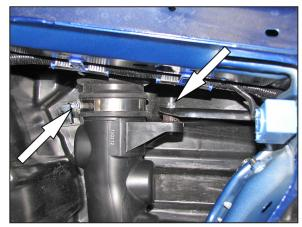
6. Loosen the hose clamp securing the intake tube and remove the nut on the lower mount. NOTE: The hose clamp may be difficult to loosen because of its position; if necessary the lower valance panel under the car may be removed for easier access.
