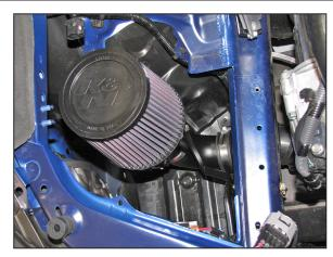
12. Install the intake tube assembly into the turbo inlet tube. Secure the tube to the mounting bracket and intake tube with the provided hardware and hose clamp.
