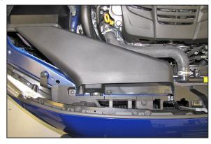
18. Install the fresh air intake scoop and secure with the factory retaining clips.
