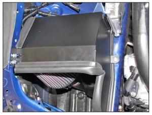
17. Install the heat shield and secure to the upper air filter housing with the factory nuts removed in step #3 and to the rubber mounted stud with the provided hardware.
