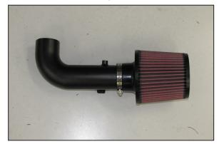
10. Install the K&N<sup>®</sup> air filter onto the K&N<sup>®</sup> intake tube and secure it with the provided hose clamp. **NOTE: Drycharger<sup>®</sup> air filter wrap; part # RX-4990DK is available to purchase separately.**
