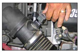
2. Depress the locking tab and disconnect the mass air sensor electrical connection.
