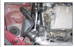
24. Install the mass air sensor and heat shield assembly. Secure with the provided hose clamp as shown.
