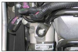
20a. On vehicles equipped with the above style heater hose tube, remove the mounting bolt shown. **NOTE: This bolt will be reused in a later step**
