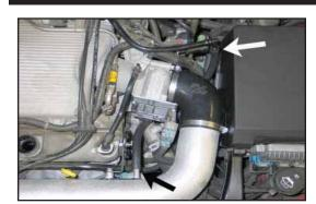
25. Cut the end of the crank case vent line, then install the provided silicone vent line onto the stock vent line and then onto the K&N Intake Tube as shown.
