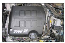
3. Remove the oil filler cap. Pull up firmly on the engine cover, removing it from the vehicle.
