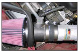
28. Re-connect the mass air sensor as shown.
