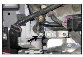
20. On vehicles equipped with the above style heater hose tube, remove the mounting bolt shown.
