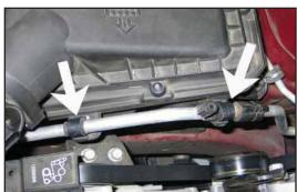
8. Remove the two clamps securing the A/C line to the stock air box.
