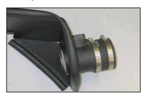
18. Install silicone hose (#08690) onto the mass air sensor with the provided hose clamp as shown.
