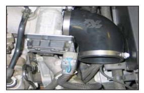
14. Install the provided silicone hose (08629) onto the throttle body with the provided hose clamp.
