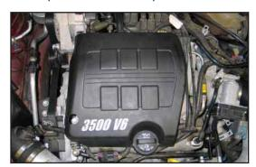
27. Install the engine cover and oil filler cap as shown.
