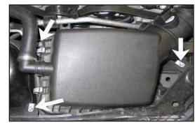
9. Remove the three bolts that secure the stock air box. On vehicles equipped with air injection, release the retaining clips and unhook the air injection hose from the air box lid.
