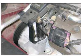
21. Install the correct tube mounting bracket (06496 or 070049) to match the style heater hose tube as shown in the above photos and secure with the factory bolt removed in step #20a.
