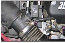
5. Loosen the hose clamp that secures the stock intake to the mass air sensor.
