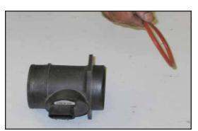
13. Remove the O-ring from the mass air sensor.
