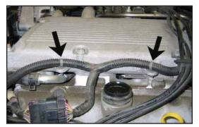
11. Remove the two clips that secure the mass air sensor harness to the upper intake plenum.
