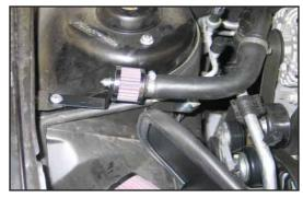
26b. Secure the air injection filter assembly to the air box mount with the provided hardware and then attach the air injection hose to the filter and secure with the provided hose clamp as shown.
