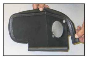
17. Install the provided edge trim (long) onto the heat shield as shown.
