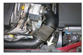
Loosen the hose clamp that secures the stock intake tube to the throttle body. Remove the bolt that secures the stock intake tube to the core support.
