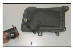
12. Remove the two Torx screws that secure the mass air sensor to the stock air box.
