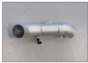
33. Install the provided 90° vent fitting into the passenger side K&N® intake tube (27620) as shown.
