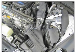
9. Disconnect the driver side mass air sensor electrical connection and unhook the wiring harness from the air box.
