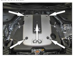
2. Remove the three bolts and two nuts securing the decorative engine cover and then remove the engine cover.
