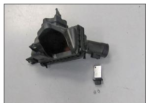
34. Remove the two screws securing the driver's side mass air sensor into the air box and then remove the sensor.
