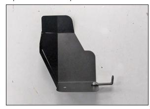
15. Install the mounting bracket (070109) onto the passenger side heat shield (073171) as shown and secure with the provided hardware.
