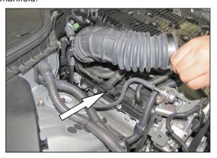
8. Pull the intake hose up to gain access to the crank case vent to valve cover connection. Release the clamp securing the crank case vent and then remove the passenger intake hose assembly.
