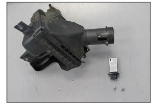
20. Remove the two screws securing the passenger side mass air sensor into the air box and then remove the sensor.
