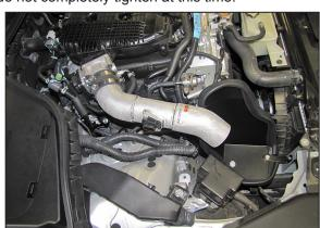
25. Install the Passenger side K&N® intake tube assembly into the coupling hose at the throttle body and the crank case vent hose onto the valve cover port. Align the mounting bracket with the hole in the heat shield and secure with the provided hardware. Do not completely tighten the mounting points at this time.
