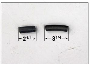
22. Cut the provided crank case vent hose into two sections as shown. One section is to be 2-1/4" long; the other section is to be 3-1/4" long.
