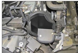
19. Install the provided straight vent fitting into the passenger side K&N® intake tube (27620) as shown.
