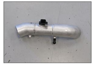
35. Install the mass air sensor into the K&N $^{\!0}$  intake tube and secure with the provided hardware.
