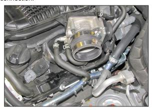
28. Install the remaining coupling hose (08440) onto the driver's side throttle body and secure with the provided hose clamp.
