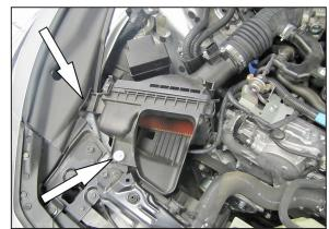
5. Remove the two bolts that secure passenger side air box and loosen the hose clamp to the
