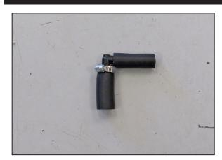
36. Install the 5/8" and  $\frac{1}{2}$ " crank case vent hose's onto the  $\frac{1}{2}$ "  $90^{\circ}$  fitting.
