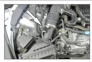
4. Disconnect the Passenger side mass air sensor electrical connection and unhook the wiring harness from the air box.
