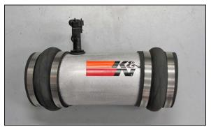
15. Install both of the coupling hoses (08418) onto the K&N^ $\ensuremath{^\circ}$  intake tube as shown.
