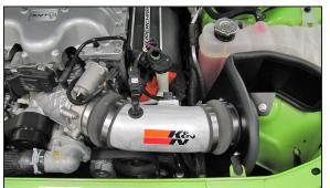
16. Install the K&N<sup>®</sup> intake tube assembly into position, Slide the coupling hoses out and onto the throttle body and filter adapter. Then adjust the tube and hoses for proper fit and secure with the provided hose clamps.
