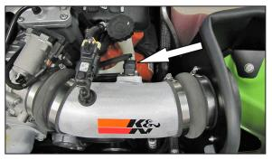
18. Reconnect the mass air sensor electrical connection.
