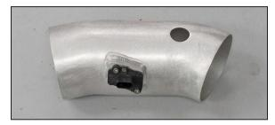
13. Install the mass air sensor into the K&N $^{\odot}$  intake tube and secure with the provided hardware.
