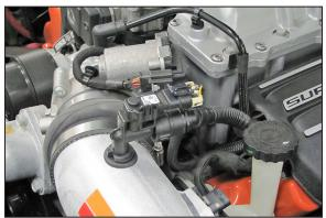
17. Reconnect the crank case vent hose and pressure sensor electrical connection. NOTE: Rotate the K&N<sup>®</sup> intake tube towards the rear of the vehicle and slide it towards the throttle body to provide the maximum amount of hood clearance, additional clearance can be achieved by rotating the crank case vent hose to adjust its position. 3. If road test is fine, you can now enjoy the added power and performance from your kit.
