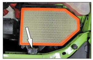
6. Remove the bolt securing the lower air filter housing to the core support and then remove the air filter housing from the vehicle. **NOTE:** It may be helpful to separate the fresh air duct from the air filter housing to aid its removal. The factory bolt will be reused in a later step. On Charger models, the fresh air intake duct stays inside the vehicle. **NOTE:** K&N Engineering, Inc., recommends that customers do not discard factory air intake.
