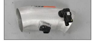
14. Install the provided grommet and pressure sensor/vent assembly into the  $K\&N^{\textcircled{s}}$  intake tube as shown.
