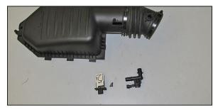
12. Remove the two screws securing the mass air sensor into the air filter housing and then remove the mass air sensor. Remove the pressure sensor/ vent assembly from the factory intake hose as shown.
