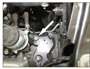
18. Remove the power steering reservoir mounting bolt shown.
