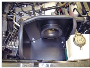
16. Set the heat shield into position on the rubber mounted studs and then secure with the provided hardware.
