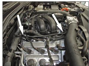
32. Connect the provided fuel pressure vent hose to the fuel pressure regulator and then connect the open end to the fitting installed into the K&N® intake tube.
