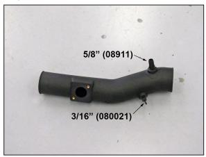
25. Install the provided vent fittings into the K&N® intake tube as shown.
