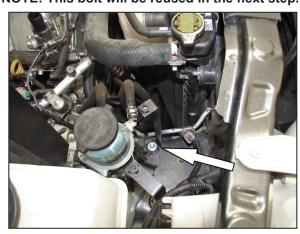
19. Install the provided secondary air pump mounting bracket (083168) onto the power steering reservoir using the bolt from the previous step.
