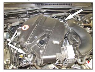
10. Remove the two bolts securing the air filter housing to the engine and then remove the air filter housing from the engine.
