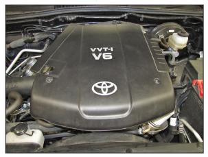
36. Install the engine cover and secure with the factory retaining nuts.
