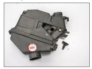
27. Remove the two screws securing the mass air sensor into the air filter housing and then remove the mass air sensor from the housing.
