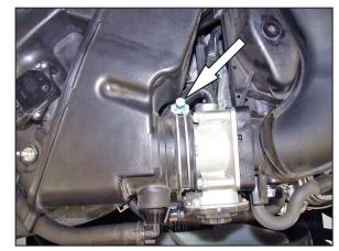
7. Loosen the hose clamp securing the intake hose to the throttle body.
