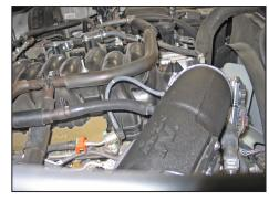
25. Connect the crank case vent hose and the fuel pressure hose to the fittings connected to the K&N® intake tube.
