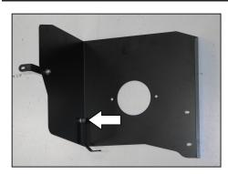
10. Install the heat shield mounting bracket (07190) onto the heat shield using the provided spacer and hardware.
