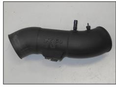
21. Install the provided NPT vent fittings into the  $K\&N^{\text{@}}$  intake tube as shown.
