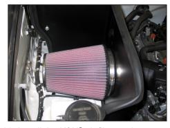
26. Install the  $K\&N^{\scriptsize @}$  air filter and secure with the provided hose clamp.
