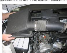
6. Release the four retaining clips securing the upper air box and then remove the upper air box and intake tube assembly from the vehicle.
