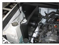
14. Set the heat shield into the engine compartment and secure the factory nuts and with the provided hardware.
