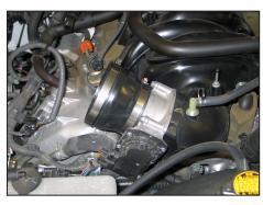
15. Install the silicone hose (08497) onto the throttle body and secure with the provided hose clamp.
