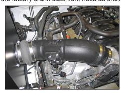
24. Insert the K&N® intake tube into the hump hose attached to the heat shield and then into the step hose attached to the throttle body. Secure with the provided hose clamps.
