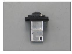
19. Install the mass air sensor through the K&N® mass air sensor adapter as shown. Secure using the provided hardware.
