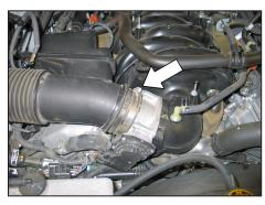
4. Loosen the hose clamp that secures the intake tube to the throttle body.
