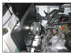
16. Install the silicone hump hose (08418) onto the filter adapter and secure with the provided hose clamp.
