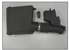
17. Remove the two screws securing the mass air sensor and then remove the mass air sensor from the upper air box housing.
