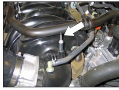
31. Install the factory mounting stud into the nut extension as shown.
