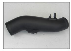
24. Install the provided NPT vent fittings into the  $K\&N^{\scriptsize @}$  intake tube as shown.
