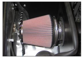
29. Install the filter assembly onto the K&N® intake tube and secure with the provided hose clamp.
