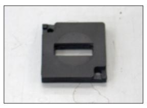
20. Install the provided gasket onto the bottom of the  $K\&N^{@}$  mass air sensor adapter as shown.
