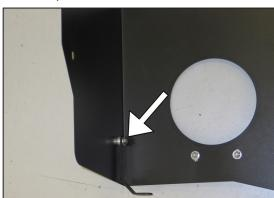
13. Install the provided heat shield mounting bracket (07190) onto the heat shield using the provided hardware and spacer as shown.
