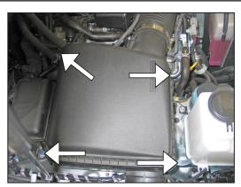
7. Release the four laches's securing the upper airbox to the lower airbox.
