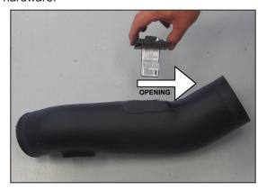
23. Install the mass air sensor assembly into the K&N® intake tube as shown using the provided hardware.
