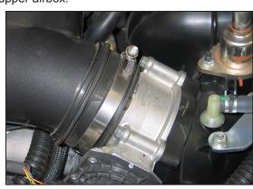
6. Loosen the hose clamp that secures the factory intake tube to the throttle body.
