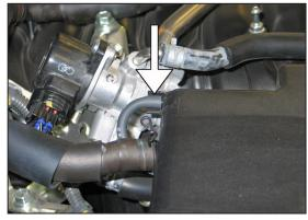
3. Disconnect the fuel pressure regulator vacuum hose from the intake tube.
