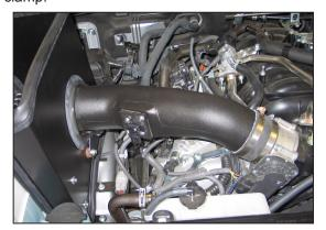
26. Install the K&N® intake tube assembly into the silicone hose at the throttle body and align with the tube mounting bracket on the heat shield. Secure the tube with the provided hardware and hose clamp.
