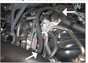
31. Install the provided crankcase vent line onto the NPT fitting installed into the K&N® intake tube and connect the open end onto the factory Tee.
