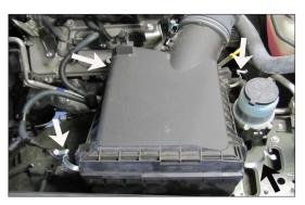
8. Release the four clips which secure the upper air box to the lower air box and then remove the intake tube and upper air box from the vehicle.
