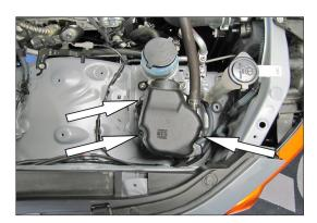
11. On models with the Air injection pump located in front of the air box next to the Power steering reservoir, remove the three bolts securing the pump to the inner fender.
