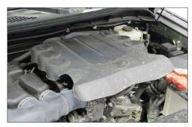
2. Lift up the engine cover to dislodge it from the mounting grommets and then remove the cover from the vehicle.
