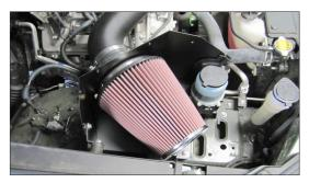
31. Install the K&N® air filter onto the filter adapter and secure with the provided hose clamp.
