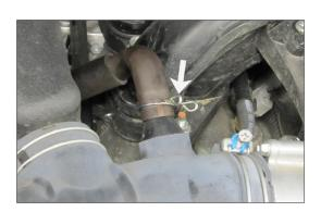
5. Disconnect the crank case vent hose from the stock intake tube.
