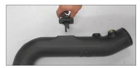
25. Install the mass air sensor assembly into the K&N® intake tube and secure with the provided hardware.
