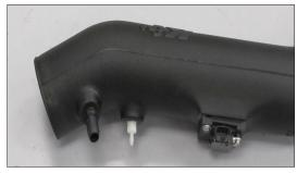
27. Install the 3/16 vent fitting into the  $K\&N^{\mbox{\scriptsize 0}}$  intake tube as shown.
