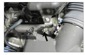
6. Remove the bolt which secures the tube mounting bracket to the engine valve cover.
