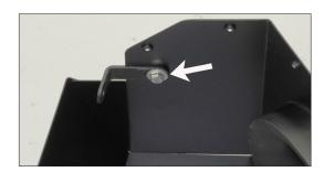
16. Install the provided mounting bracket (08022) onto the heat shield and secure with the provided hardware.
