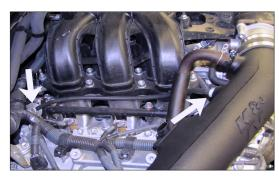
30. Connect the provided fuel pressure vent line to the fuel pressure regulator and then connect the open end to the 3/16 vent fitting in the K&N® intake tube.
