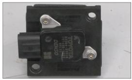
24. Install the mass air sensor into the K&N® mass air sensor adapter and secure with the provided hardware.
