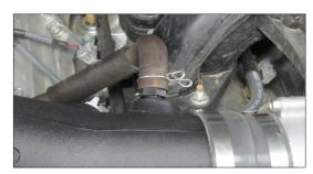
29. Connect the crank case vent line to the 5/8 vent fitting and secure with the factory spring clamp.
