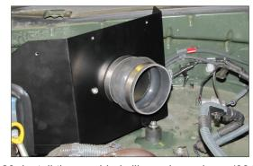
20. Install the provided silicone hump hose (084057) onto the filter adapter and secure with the provided hose clamp.
