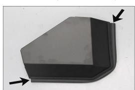
32. Install the remaining 19" piece of edge trim onto the heat shield cover as shown.
