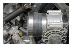
21. Install the provided silicone step hose (084091) onto the throttle body and secure with the provided hose clamp.
