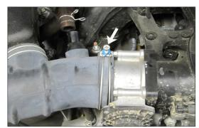
7. Loosen the hose clamp which secures the intake tube to the throttle body.
