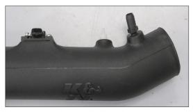
26. Install the 5/8 vent fitting into the K&N® intake tube as shown.
