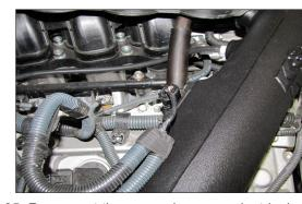
35. Reconnect the mass air sensor electrical connection.
