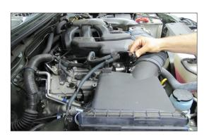
3. Disconnect the mass air sensor electrical connection and then unhook the wiring harness from the air box.
