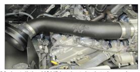
28. Install the K&N® intake tube into hump hose at the filter adapter and then into the silicone hose at the throttle body, align the tube for proper fit and then tighten the hose clamps.
