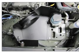
19. Set the heat shield onto the rubber mounted studs and the secure with the provided hardware. NOTE: On models that had a horn attached in this location, be sure to reattach the horn between the heat shield bracket and rubber mounted stud.
