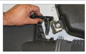
23. Remove the screws which secure the mass air sensor to the factory air box and then remove the mass air sensor from the air box.
