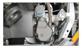
19a. Install the air injection pump onto the heat shield and forward rubber mounted stud and then secure with the provided hardware. Reconnect the air injection pump electrical connection.
