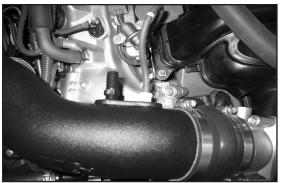
26. Connect the factory fuel pressure vent hose to the intake tube as shown.
