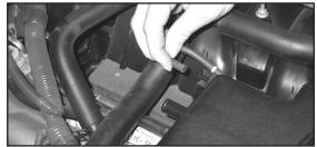
5. Disconnect the fuel pressure regulator vent hose from the factory intake tube as shown.
