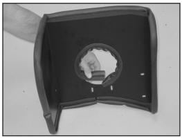
10. Install the small edge trim into the hole of the heat shield as shown.
