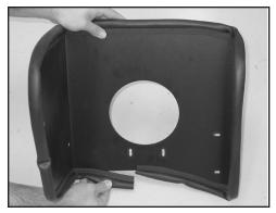
9. Install the large edge trim onto the heat shield as shown.
