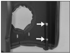
11. Install the large "L" bracket (#070902) onto the heat shield using the provided hardware and spacers as shown.
