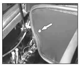
18. Secure the rear heat shield bracket (installed in step #14) to the heat shield with the provided spacer and hardware.
