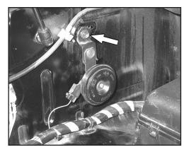
13. On vehicles equipped with a security system horn, remove the bolt that secures the horn to the inner fender.
