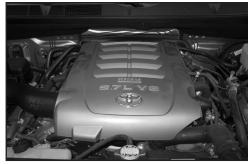
32. Re-install the engine cover onto the engine.
