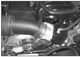
6. Loosen the hose clamp that secures the factory intake tube to the throttle body.
