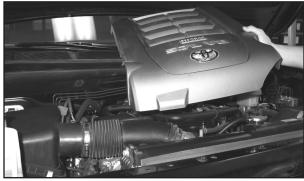
2. Lift the front of the engine cover up, then un-hook it from the rear. Remove it from the vehicle.
