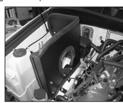
16. Set the heat shield into position on the inner fender. Then, secure the front mounting bracket to the front air box mounting location with the provided hardware.
