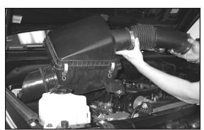
8. Remove the complete factory intake system from the vehicle.
