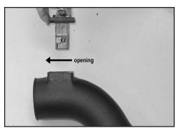
22. Install the mass air sensor assembly into the intake tube and secure with the provided hardware as shown.
