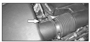
3. Disconnect the mass air sensor electrical connection. Un-hook the wiring harness from the air box.
