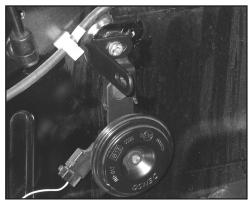
14. Install the small "L" bracket (#070742) onto the inner fender using the provided hardware as shown.
