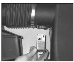
20. Remove the two bolts that secure the mass air sensor into the stock air filter housing. Remove the mass air sensor as shown.
