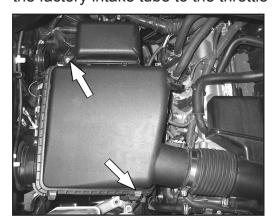
7. Loosen the two bolts that secure the air box to the inner fender.
