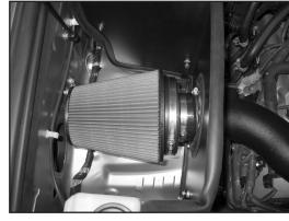
31. Install the K&N<sup>®</sup> air filter assembly onto the intake tube and secure with the provided hose clamp.
