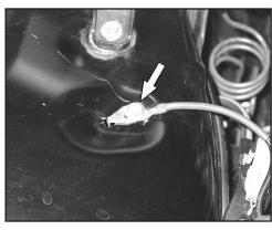
15. Remove the bolt that secures the ground strap to the inner fender.
