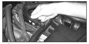
4. Disconnect the crank case vent hose from the factory intake tube as shown.
