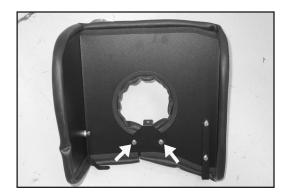
12a. Install the tube mounting bracket onto the heatshield as shown using the provided hardware.
