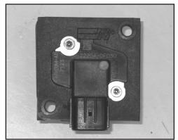
21. Install the mass air sensor into the mass air sensor adaptor and secure with the provided hardware.
