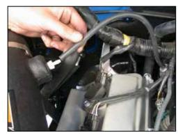
28. Install the supplied fuel pressure regulator vent hose onto the fuel pressure regulator. Attach the opposite end of the vent hose onto the K&N® intake tube as shown.
