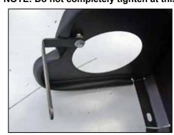
14. Install the "L" bracket onto the heat shield using the supplied spacer between the heat shield and bracket.
