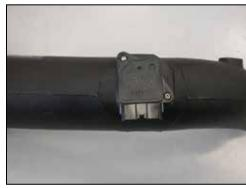
21. Install the mass air sensor assembly into the  $K\&N^{\otimes}$  intake tube using the supplied hardware.
