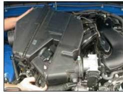
9. Lift up and remove the airbox assembly from the engine.
