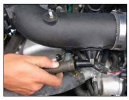
29. Install the crankcase vent hose onto the vent fitting and secure with the factory clamp.
