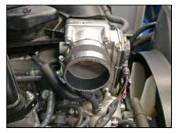
26. Install the silicone hose (08434) onto the throttle body and secure with the provided hose clamp.
