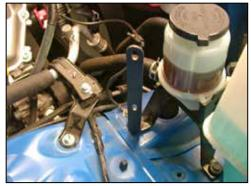
13. Install the "L" bracket onto the power steering reservoir using the bolt removed in step #12. **NOTE: Do not completely tighten at this time.**
