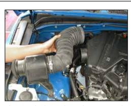
7. Loosen the hose clamp that secures the intake tube to the stock air filter housing, then remove the intake tube and resonator assembly.
