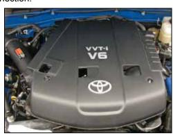
34. Reinstall the engine cover and secure with the factory nuts.
