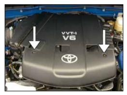
2. Loosen the two nuts that secure the engine cover.
