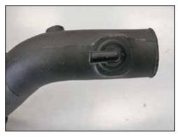
23. Install the stock crankcase vent fitting into the grommet that was installed in the K&N® intake tube in the previous step.
