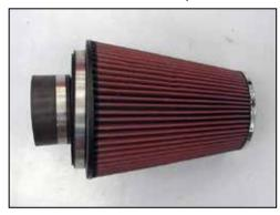
31. Install the supplied silicone hose (08630) onto the K&N® air filter assembly and secure with the provided hose clamp.
