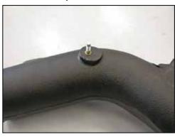
25. Install the engine cover mounting stud into the K&N® intake tube as shown, this stud was removed in step #19.
