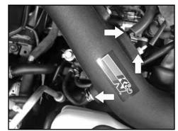
20. Install the supplied crank case vent and fuel pressure regulator vent hose's onto the engine and connect to the K&N<sup>®</sup> intake tube as shown. Connect the factory power steering pressure switch vent onto the K&N intake tube.
