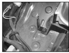
8. Remove the 12mm bolt that retains the power steering reserve to vehicle then mount the provided bracket (07158) onto the vehicle with the bolt that was removed.
