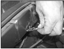
24. Disconnect the ground strap that's attached to the mass air sensor wiring harness at the inner fender as shown.
