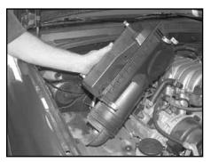
7. Remove the three bolts that retain the air box to vehicle, then remove the air box. NOTE: K&N recommends that customers do not discard factory air intake. 9. Mount the two provided brackets onto the vehicle with the provided hardware. **NOTE: Bracket (07172) mounts closest to engine.**
