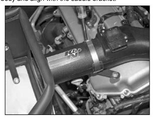
28. Secure the K&N® intake tube to the saddle bracket with the provided hose clamps also tighten the hose clamp at the throttle body.
