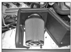
31. Install the K&N<sup>®</sup> Air filter onto the intake tube as shown.
