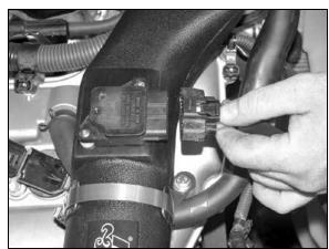
32. Reconnect the mass air sensor electrical connections.
