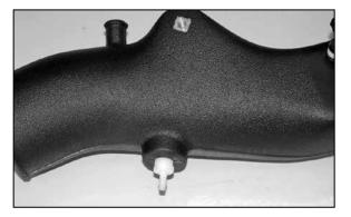
25. Install the vent fitting onto the  $K\&N^{\otimes}$  intake tube as shown.
