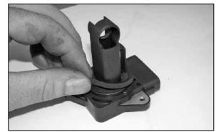
23. Apply the gasket to the mass air sensor, sticky side down as shown.
