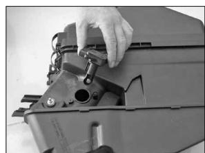
22. Remove the two screws that secure the mass air sensor to the air box assembly, then remove the mass air sensor as shown.
