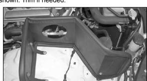
17. Install the heat shield onto the vehicle, then secure to brackets with the provided hardware.
