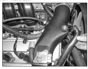
30. Fuel pressure regulator and then onto the K&N® intake tube. Install the original crank case vent hose onto the valve cover, then connect the crank case vent hose onto the K&N® intake tube.
