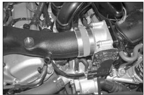
27. Install the K&N® intake tube onto the throttle body and align with the saddle bracket.
