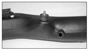
26. Install rubber mounted stud onto  $K\&N^{\otimes}$  intake tube as shown.
