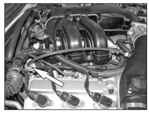
29. Remove the stock vacuum hose from fuel pressure regulator, then install provided silicone hose to fuel pressure regulator and then onto the K&N® intake tube.
