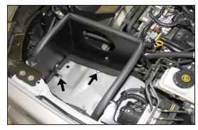
19. Install the heat shield assembly into the vehicle and secure with the provided hardware.
