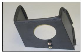
16. Install the provided rubber mounted studs onto the heat shield using the supplied hardware.
