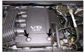
3. Remove the two bolts shown, which secure the engine cover.
