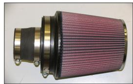
26. Install the silicone hose (08698) onto the air filter as shown and secure with the provided hose clamp.
