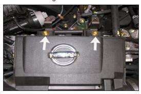
5. Remove the two bolts shown which secure the stock intake tube to the engine.
