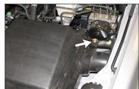
9. Remove the air box retaining bolt shown.
