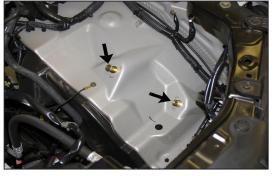
11. Remove the two air box mounting studs shown from the inner fender.
