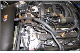
24. Attach the provided silicone crank case vent hose to the valve cover and K&N® intake tube as shown.
