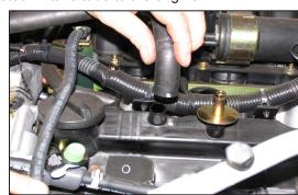
6. Using pliers, loosen the spring clamp which secures the crank case vent hose to the valve cover and then remove the hose from the valve cover as shown.
