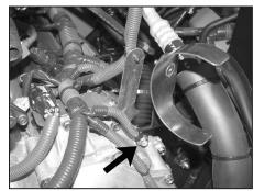
17. Install the saddle bracket assembly and ground wire removed in step #16 with the provided hardware as shown.
