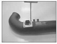
23. Secure the mass air sensor assembly onto the  $K\&N^{\mbox{\tiny @}}$  intake tube with the provided hardware.
