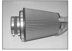
29. Install the filter adapter assembly into the  $K\&N^{\circledast}$  air filter.
