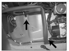
14. Install the heat shield onto the vehicle and secure with the provided hardware. **NOTE: On four wheel drive vehicles, insert differential vent retaining clip into the hole provided on the heat shield.**
