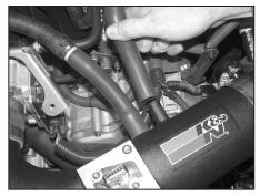
27. Install the provided silicone hose onto the hose mender, then install the hoses onto the intake tube as shown.
