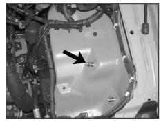
9. Remove the air box mounting stud shown with a 10mm wrench.
