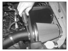
30. Install the K&N<sup>®</sup> air filter assembly onto the K&N<sup>®</sup> intake tube as shown; secure with the provided hose clamp.
