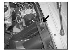
7. Remove the air box mounting bolt with a 10mm socket.
