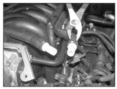
26. Install the provided hose mender into the two crank case vent hoses and secure the existing spring clamps as shown.
