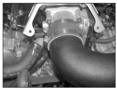
24. Install the K&N<sup>®</sup> intake tube onto the throttle body and align with the saddle bracket.
