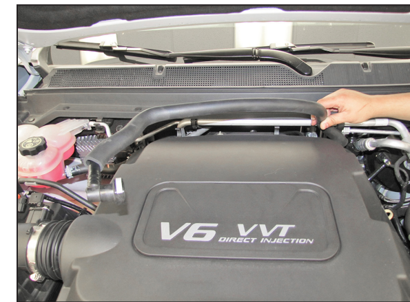
3. Disconnect the crank case vent hose from the intake plenum and then disconnect it from fitting on the valve cover.
