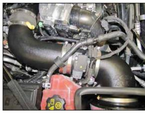
19. Connect the provided Mass air sensor extension harness into the factory harness and then reconnect the Mass air sensor and humidity sensor electrical connections.
