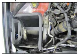
9. Install the K&N® heat shield onto the air box mounting plate tabs and secure with the three of the bolts removed in step #7.
