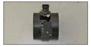
14. Install the sensors into the K&N<sup>®</sup> Mass air sensor housing and secure with the provided hardware.
