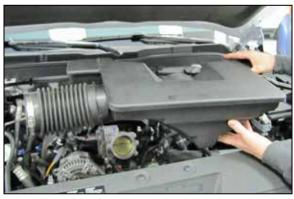
5. Remove the intake plenum from the vehicle.
