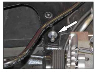
9. Remove the air box mounting stud from the inner fender.
