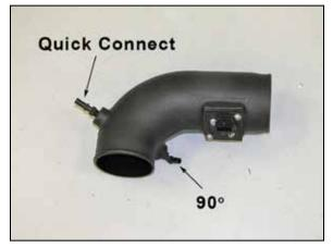
24. Install the provided vent fittings into the into the K&N® intake tube as shown.
