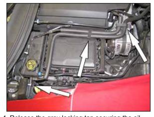
4. Release the grey locking tap securing the oil tank vent hose to the oil tank, then unhook the oil tank vent hose from the two retaining clips and remove the hose from the vehicle.
