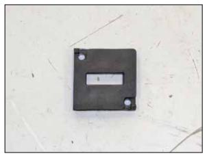
21. Install the provided gasket onto the K&N® mass air sensor adapter as shown.
