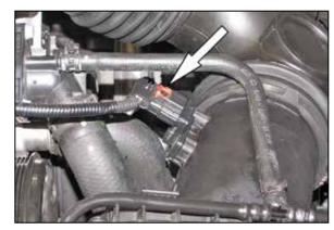
5. Disconnect the mass air sensor electrical connection.
