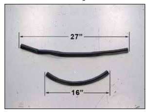
15. Cut the provided edge trim into two sections. One section should be 16" long, one section should be 27" long.
