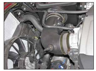
25. Install the K&N® intake tube assembly into the air filter coupling hose and then into the coupling hose at the throttle body. Adjust the tube and filter for best fit and then secure with the provided hose clamps.
