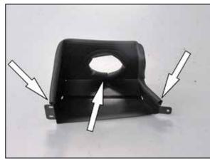
16. Install the 16" section into the hole of the heat shield and install the 27" section around the perimeter of the heat shield as shown.
