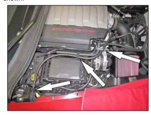
28. Install the crank case vent hose assembly onto the oil tank and then route it through the factory retaining clips and then connect the open end to the 90° fitting installed into the K&N® intake tube. NOTE: Some trimming of the hose may be necessary.
