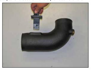
23. Install the mass air sensor assembly into the K&N® intake tube and secure with provided hardware.
