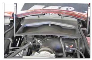
30. Reinstall the air extraction duct and secure with the factory hardware.
