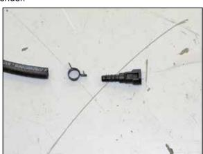
10. Assemble the provided coolant hose (08636), quick disconnect fitting and clamps. Install one clamp 1.5" from the open end of the provided coolant hose.
