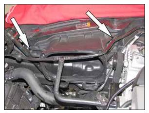
8. Remove the two bolts that secure the air filter housing to the inner fender then unhook the housing from the mounting stud and remove the housing from the vehicle.
