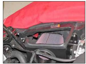
18. Install the heat shield assembly onto the rubber mounted studs and secure with the provided hardware.
