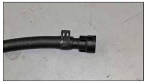
27. Assemble the provided crank case vent hose (08635) and quick disconnect fitting and clamp as shown.
