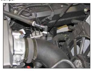
26. Connect the crank case vent hose to the fitting installed into the K&N® intake tube as shown.
