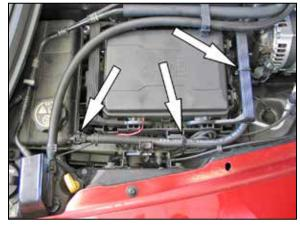
13. Install the provided coolant hose assembled from step #10 onto the expansion tank. Route the coolant hose and then attach the open end onto the TEE fitting and secure with the provided spring clamp. Use the provided tie wraps to secure the coolant hose.
