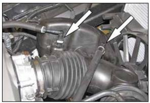
3. Release the grey locking tabs securing the crank case vent and oil tank vent tubes to the factory intake hoses and then disconnect the crank case hoses from the intake tube.
