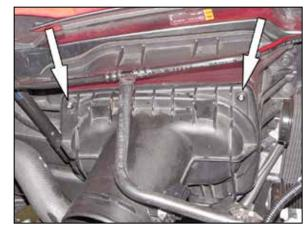
7. Loosen the two TORX fasteners securing the factory mass air sensor housing the air filter housing and then remove the mass air housing and air filter from the vehicle.
