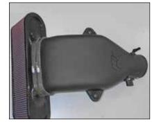
16. Install the K&N® air filter onto the K&N® intake tube as shown and secure with the provided hose clamp.
