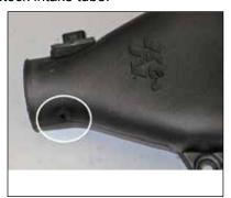
11. Install the provided grommet into K&N® intake tube as shown.
