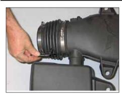
10. Remove the crankcase vent fitting from the stock intake tube.
