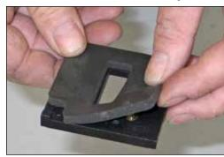
6. Install the provided gasket onto the mass air sensor adapter as shown.
