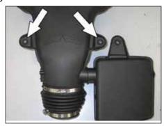
13. Remove the two intake tube mounting grommets from the stock intake tube.
