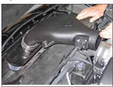
18. Install the K&N® intake assembly on top off the radiator assembly and then connect the mass air sensor electrical connection as shown.
