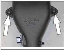
14. Install the two mounting grommets into the  $K\&N^{\otimes}$  intake tube.
