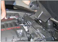
5. Lift up and remove the complete stock intake system from the vehicle as shown.
