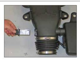
7. Remove the two screws which secure the mass air sensor to the stock intake tube and then remove the mass air sensor from the intake tube as shown.
