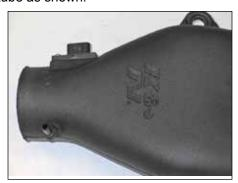
12. Install the factory crankcase vent fitting into the grommet as shown.
