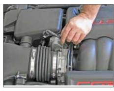
2. Unlock and disconnect the crankcase vent tube from the intake tube as shown.
