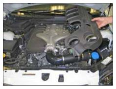
21. Remove the driver's side engine cover as shown.
