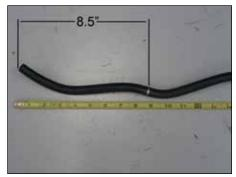
24. Measure 8.5' from the end of the tube and then cut the tube using a sharp knife.
