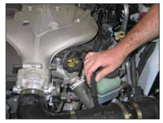
26. Install the crank case breather hose onto the valve cover and connect the open end to the vent fitting attached to the K&N® intake tube.
