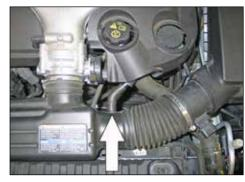
3. Disconnect the crank case vent line from the factory intake tube.
