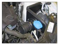
16. Install the mass air sensor onto the heat shield assembly and secure with the provided hose clamp. NOTE: Be sure to correctly position the mass air sensor in the correct direction as indicated by the arrow which shows the way of air travel.
