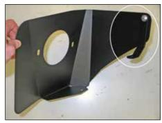
9. Install the heat shield mounting bracket (07190) onto the heat shield as shown using the provided hardware.
