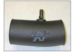
17. Install the 1/4" npt vent fitting into the K&N® intake tube as shown.
