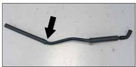
25. Install the provided silicone hose onto the factory crank case vent tube as shown.
