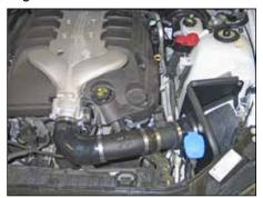
14. Install the heat shield assembly into the vehicle and secure with the factory nut from step #6 and hardware provided.
