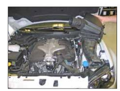
7. Pull up firmly and remove the air box from the vehicle.
