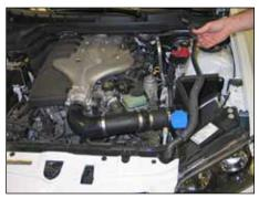
22. Disconnect the crank case vent tube from the valve cover and remove from the vehicle.
