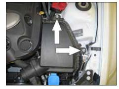
6. Remove the two nuts which secure factory air box to the inner fender.
