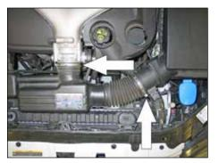
4. Loosen the hose clamps which secure the factory intake tube to the mass air sensor and throttle body.
