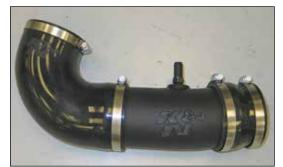
19. Install the silicone hose (08051) onto the K&N® intake tube and secure with the provided hose clamp.
