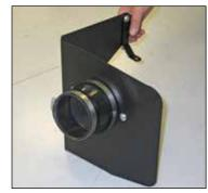
11. Install the provided silicone hose (08050) onto the filter adapter and secure with the provided hose clamp.
