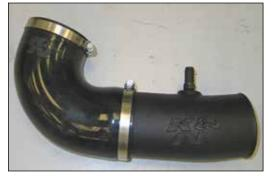
18. Install the angle hose (084089) onto the K&N® intake tube and secure with the provided hose clamp.
