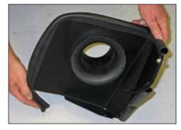
13. Install the longer edge trim onto the heat shield as shown.
