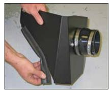
12. Install the shorter edge trim onto the heat shield as shown.
