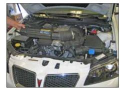
5. Remove the intake tube from the vehicle
