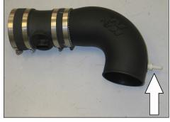
20. Install the crankcase fitting into the  $K\&N^{\circledast}$  intake tube as shown.
