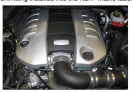
24. Remove the oil fill cap and reinstall the engine cover. Reinstall the oil fill cap.
