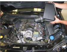
8. Remove the complete air box assembly from the
