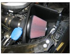
25. Install the air filter and secure with the provided hose clamp.
