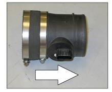
16. Loosen the hose clamp and remove the mass air sensor from the factory air box. Install the provided silicone hose (08761) onto the mass air sensor and secure with the provided hose clamp. NOTE: Note the air flow direction of the mass air sensor by the arrow embossed on the side.
