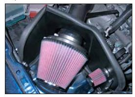
24. Install the air filter assembly onto the K&N<sup>®</sup> intake tube and secure with the provided hose clamp.
