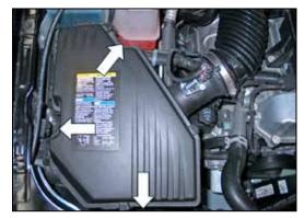
4. Loosen and remove the two air box mounting bolts and one mounting nut as shown. NOTE: 2008 and and later vehicles are not equipped with the retaining nut. All other vehicles will use the retaining nut in a later step.
