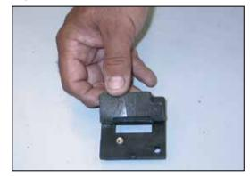
13. Install the provided gasket onto the K&N $^{\mbox{\tiny \$}}$  mass air sensor adapter as shown.
