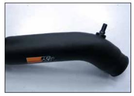
17. Install the provided  $1\!\!\!/4"$  NPT fitting into the K&N® intake tube as shown.
