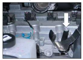
19. Install the tube mounting bracket assembly onto the valve cover. Place the provided large spacer between the bracket and valve cover, and secure with the factory bolt removed in step #6 as shown.
