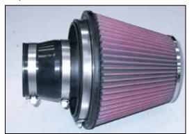
23. Install the silicone hose (#08724) onto the air filter adapter and secure with the provided hose clamp.
