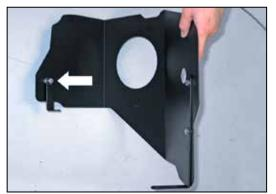
10. Install the small "L" bracket (#070602) onto the heat shield with the provided hardware as shown. **NOTE: Use one of the provided spacers between the bracket and heat shield.**
