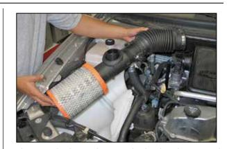
7. Loosen the hose clamp at the intake plenum and then remove the complete intake system. NOTE: K&N Engineering, Inc., recommends that
