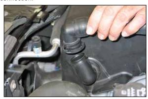
3. Depress the locking tabs and disconnect the air injection hose.
