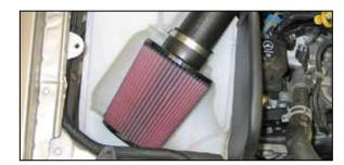
20. Install the K&N® air filter onto the K&N® intake tube and secure with the provided hose clamp. NOTE: Drycharger® air filter wrap; part # RX-4730DK is available to purchase separately.
