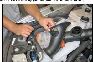
6. Remove the fresh air supply duct.
