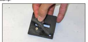
14. Install the adapter gasket onto the adapter plate as shown.
