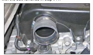
13. Install the provided silicone hose (08051) to the throttle body and secure it with the provided hose clamp.
