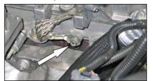
11. Remove the engine ground strap bolt shown. **NOTE: This bolt will be reused.**
