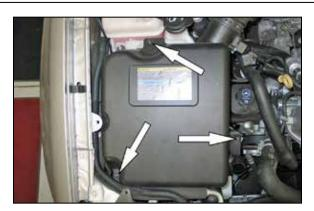
4. Loosen the three screws which secure the upper air box.
