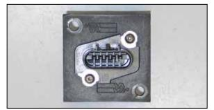
15. Install the mass air sensor into the mass air adapter and secure with the provided hardware.
