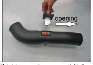
16. Install the mass air sensor assembly into the K&N<sup>®</sup> intake tube and secure with the provided hardware.
