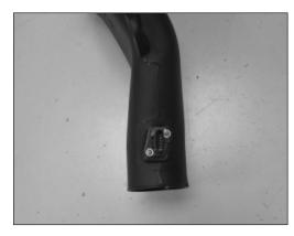
8. Secure the mass air sensor to the K&N Intake Tube with the screws and spacers provided.
