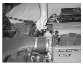
2. Unlock and disconnect the crank case vent hose from the intake tube as shown.
