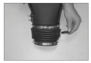
9. Remove the crank case vent fitting from the stock intake tube as shown.
