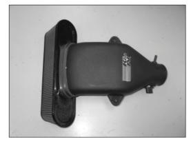
15. Install the K&N Air Filter into the silicone hose installed on the K&N Intake Tube as shown and secure with the provided hose clamp.
