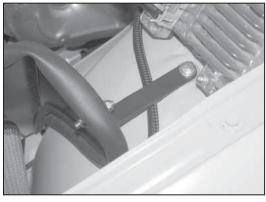
15. Install the heat shield mounting bracket onto the heat shield and secure the bracket to the inner fender at the upper air box mounting pin location with the provided hardware.
