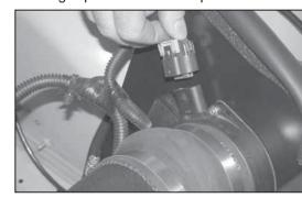
21. Reconnect the mass air sensor electrical connection.
