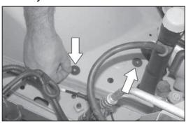
12. Place the two rubber washers onto the inner fender at the lower air box mounting pin locations as shown.
