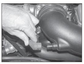
4. Disconnect the crank case vent hose from the factory intake tube as shown.
