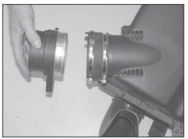
9. Loosen the hose clamp that secures the mass air sensor to the factory air box, then remove the mass air sensor from the factory air box.
