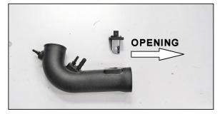
23. Install the mass air sensor assembly into the  $K\&N^{\circ}$  intake tube so that the opening in the sensor faces towards the filter end of the tube and secure with the provided hardware
