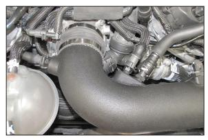
25. Connect the crank case vent, EVAP vent and idle by pass lines to the quick disconnect fittings installed into the K $\&N^{\otimes}$  intake tube.
