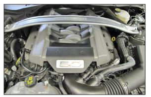
2. Lift up the decorative engine cover to dislodge it from the mounting studs and then remove the engine cover from the vehicle. 3. Depress the locking tab and then disconnect the idle bypass hose from the intake tube.
