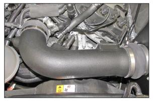
24. Install the K&N<sup>®</sup> intake tube into the hose at the filter adapter and then into the hose at the throttle body, adjust the tube for best fit and then secure with the provided hose clamps.
