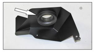
12. Install the provided filter adapter into the heat shield as shown and secure with the provided hardware.
