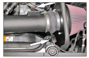
26. Connect the provided mass air sensor extension harness into the factory mass air sensor connection and then connect the other end to the mass air sensor.
