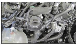
18. Install the provided hump coupler (08699) onto the throttle body and secure with the provided hose clamp. nui ule provideu naluwale.
