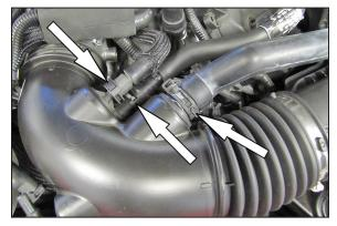
4. Depress the locking tabs and then disconnect the crank case vent hose and the EVAP vent hose. Then release the spring clamp and disconnect the sound tube from the intake tube. 5. Loosen the hose clamps securing the factory intake tube and then remove the intake tube from the vehicle.
