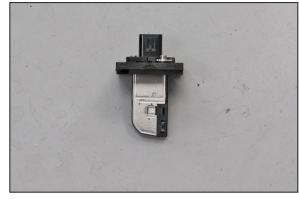
18. Install the mass air sensor into the K&N® adapter and secure with the provided hardware.
