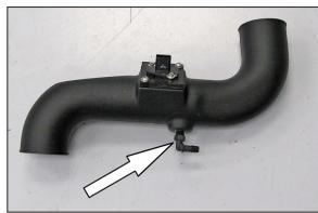
20. Install the  $90^{\circ}$  vent fitting into the K&N<sup>®</sup> intake tube as shown.
