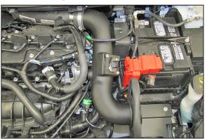
21. Install the K&N® intake tube assembly into the silicone hose at the turbo inlet pipe and then into the heat shield, adjust the tube for proper fit and then secure with the provided hose clamps.
