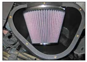
29. Install the K&N® air filter onto the filter adapter and secure with the provided hose clamp.
