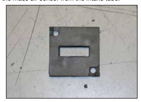
23. Install the provided mass air adapter gasket as shown.
