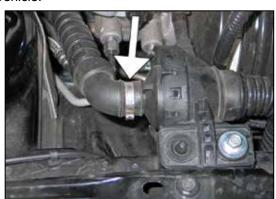
3. Cut the clamp that secures the engine pulse hose to the drum and disconnect the hose from the drum.
