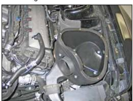
17. Set the K&N® airbox into the vehicle so that the mounting studs slide into the mounting holes, and then secure with the hardware provided.
