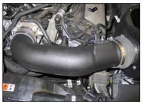
26. Install the K&N® intake tube into the silicone hose at the airbox and then into the silicone hose at the throttle body; secure with the provided hose clamps.
