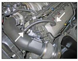
27. Install the crankcase vent hose to the fitting on the K&N® intake tube and onto the valve cover. Vehicles equipped with an EVAP vent line, connect it to the fitting installed in the K&N® intake tube.
