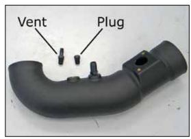
21. On vehicles that have an EVAP vent line attached to the intake tube, install the 3/8" vent fitting into the K&N® intake tube. On vehicles that do not have the EVAP vent line attached to the intake tube, install the NPT plug into the intake tube.
