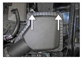
9. Release the two upper airbox retaining clips.
