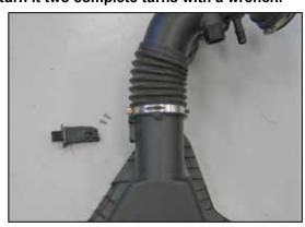
22. Remove the two bolts securing the mass air sensor into the factory intake tube and then remove the mass air sensor from the intake tube.
