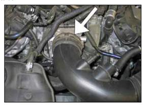
8. Loosen the hose clamp that secures the factory intake tube to the throttle body.
