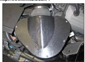
30. Install the K&N<sup>®</sup> airbox lid and secure with the provided hardware.
