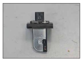
24. Install the mass air sensor into the K&N® adapter and secure with the provided hardware.
