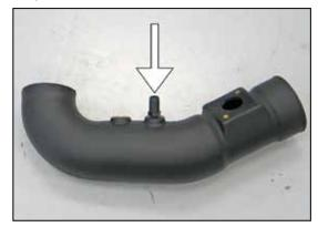
20. Install the crankcase vent fitting into the K&N® intake tube as shown.
