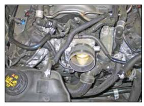
19. Install the provided silicone hose (08698) onto the throttle body and secure with the provided hose clamp.
