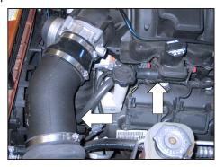
21. Install the assembled vent hose onto the fitting installed in the K&N® intake tube and then attach the open end to the valve cover port.
