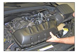
7. Remove the upper airbox and intake tube assembly.
