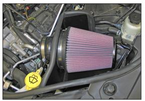
Install the K&N<sup>®</sup> filter onto the adapter and secure with the provided hose clamp.
