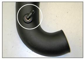
21. Install the 90° npt fitting into the K&N $^{\mbox{\tiny 8}}$  intake tube as shown.
