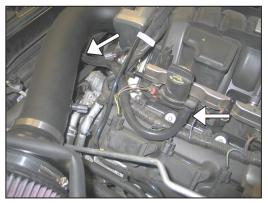
23. Install the crankcase vent hose onto the 90° vent fitting and then attach the open end to the valve cover port.
