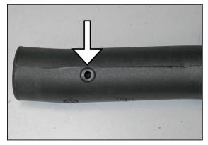
19. Install the provided grommet into the  $K\&N^{\circledast}$  intake tube as shown.
