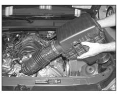
7. Lift the complete intake and air filter assembly to remove it from the vehicle.
