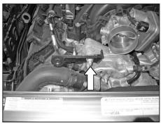
7a. On vehicles equipped with an intake resonator, remove the nut shown that secures the resonator bracket; remove the resonator bracket from the engine.
