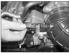
3. Unlock the red locking tab on the air temperature sensor electrical connection, then depress the locking lever and pull apart the temperature sensor electrical connection.
