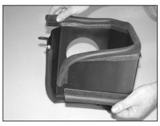
10. Install the two pieces of edge trim onto the heat shield as shown, be sure to leave a gap at the bracket mounting locations.
