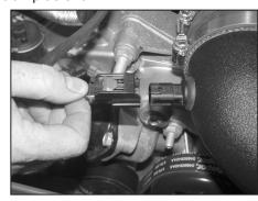
23. Reconnect the air temperature sensor electrical connection as shown.
