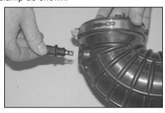
15. Remove the air temperature sensor from the factory intake tube.
