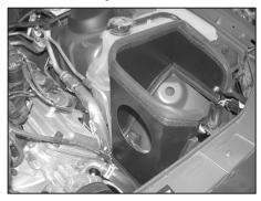
11. Install the heat shield assembly into the vehicle and secure to the bracket installed in step #8. Then secure the "L" bracket with the factory bolt removed in step #6 to the airbox mounting location.
