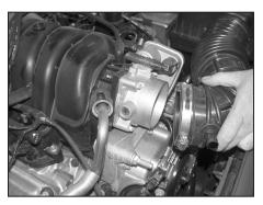
4. Loosen the hose clamp that secures the intake tube to the throttle body and pull the intake tube off of the throttle body.
