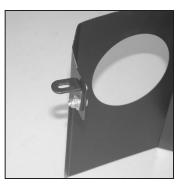
9. Install the "L" bracket (070066) onto the heat shield with the provided hardware through the non-slotted hole in the bracket.
