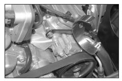
13. Using the provided spacer, install the tube mounting bracket assembly onto the engine as shown.
