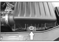
6. Loosen and remove the airbox mounting bolt as shown.
