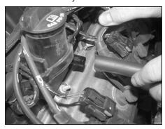
5. Disconnect the crank case vent hose from the valve cover port as shown.
