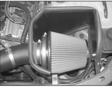
22. Install the air filter assembly onto the K&N® intake tube and secure with the provided hose clamp as shown.
