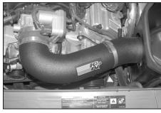
18. Install the K&N® intake tube into the throttle body and onto the saddle clamp as shown, then secure with the hose clamps provided.
