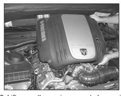
2. Lift up on the engine cover to loosen it from the mounts, and then remove the cover from the vehicle.
