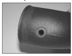
16. Install the provided grommet into the K&N<sup>®</sup> intake tube as shown.
