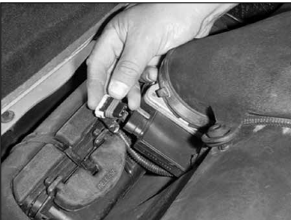
2. Disconnect the mass air sensor electrical connection.
