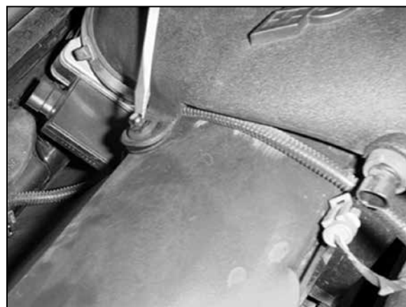
4. Release the push clips that retain the stock intake tube to the upper radiator cover.
