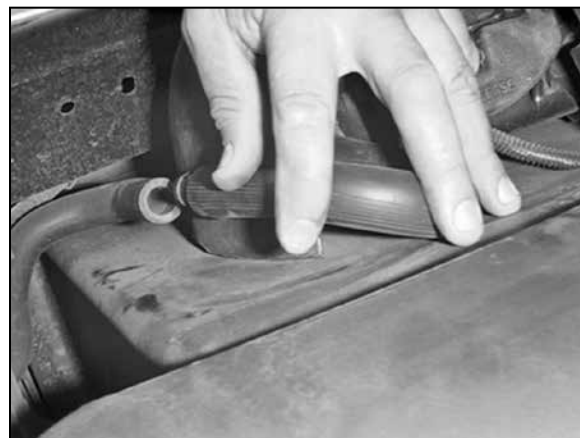
3. Disconnect the air injection vent hose.
