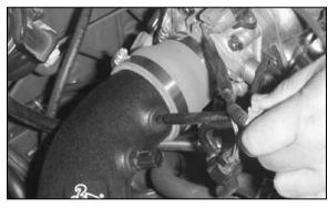
16. Insert the crankcase vent tube into the second grommet on the K&N® intake tube.
