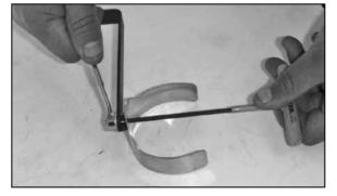
8. Assemble the saddle to the bracket as shown. NOTE: On models with manual trans. use the "L" bracket and on EX models with auto trans. use the angled "L" bracket.
