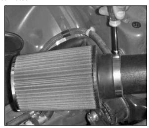
18. Install the Air Filter element onto the intake tube and secure it with the provided hose clamp.
