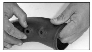
10. Install the grommets supplied into the 2 small holes in the  $K\&N^{\circ}$  intake tube.
