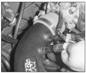
17. Reconnect the air temperature sensor electrical connection.
