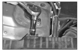
3. Loosen and remove the two bolts that secure the airbox.
