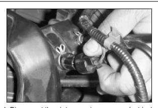
4. Disconnect the air temperature sensor electrical connection.
