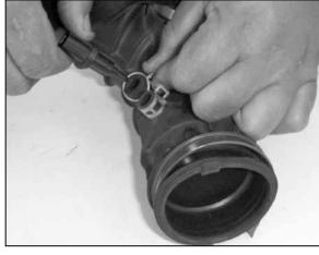
14. Remove the air temperature sensor from the stock intake tube.
