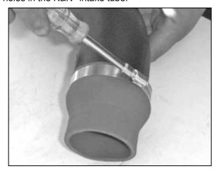
11. Install the silicone adapter onto the  $K\&N^{\scriptsize @}$  intake tube.
