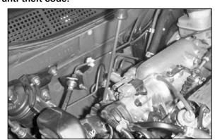
2. Loosen the hose clamp on the  $\underline{\text{intake tube}}$  at the throttle body.
