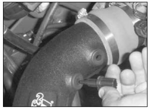
15. Install the air temperature into the grommet on the K&N® intake tube.
