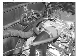
22. Remove the factory crank case vent line and replace it with the provided silicone hose and hose clamp as shown.
