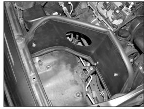
17. Using the provided hardware secure the heat shiled onto the vehicle as shown. Do not tighten completly.
