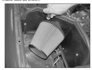
30. Install the  $K\&N^{\otimes}$  air filter onto the filter adaptor as shown.
