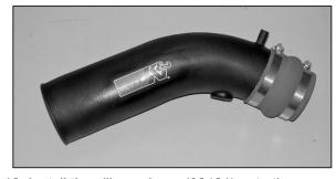
18. Install the silicone hose (08421) onto the new K&N® intake tube with the provided hose clamps.
