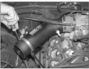
21. Install the new intake tube onto the throttle body, then secure intake tube to saddle bracket with the provided hose clamp.
