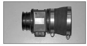
20. Install the silicone hose (08724) onto the mass air sensor with the provided hose clamps.
