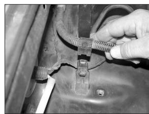
16. Disconnect the wire harness from vehicle, then locate harness on other side of bracket.
