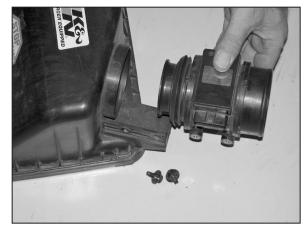
7. Remove the two bolts that secure the mass air sensor to the air box, then remove the mass air sensor as shown.
