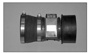
27. Install the filter adaptor onto the mass air sensor as shown.
