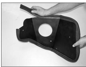
15. Install edge trim onto heat shield as shown. Trim if needed.
