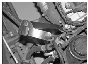
11. Install the saddle bracket assembly onto the motor using the bolt that was removed in the previous step.
