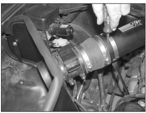
29. Install the mass air sensor onto the new  $K\&N^{\otimes}$  intake tube as shown.
