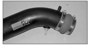
19. Install the NPT fitting onto the K&N $^{\! \rm B}$  intake tube as shown.
