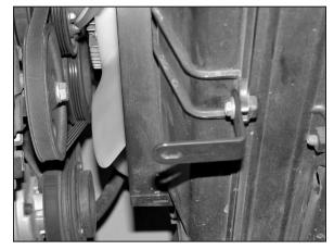
12. Remove the 10mm bolt that retains the fan shroud to radiator, then secure the provided bracket (070662) to the radiator with the bolt that was removed.
