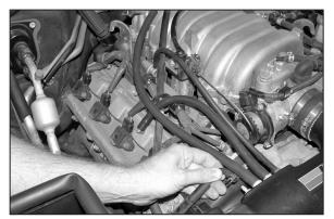
27. Install the three provided vent hoses in place of the vent hoses removed in step #9, and connect them to the vent fittings in the K&N® intake tube. Also re-connect the one existing vent hose to the vent fitting.
