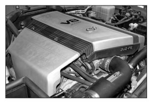
30. Reinstall the engine cover with hardware removed in step #2.
