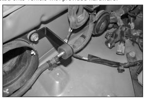
16. Remove 10mm bolt securing fresh air duct and install bracket (07093) onto vehicle with bolt that was removed.
