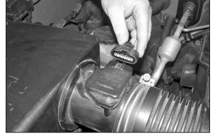
3. Disconnect the mass air sensor electrical connection and mass air sensor wire harness, retaining clip from the air box.
