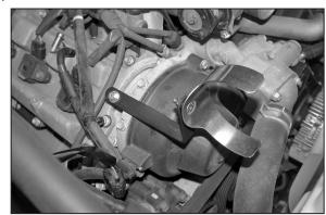
24. Install saddle bracket assembly onto cam cover with provided hardware.
