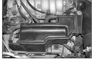
4. Remove the four vent lines from the air intake resonator as shown.
