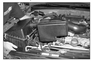
8. Remove the intake tube from the throttle body, then remove the complete air intake assembly.
