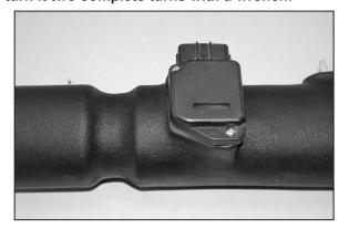
22. Install mass air sensor onto tube with provided bolts and nylon spacers as shown.
