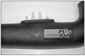
21. Install provided npt vent fittings onto tube as shown.
