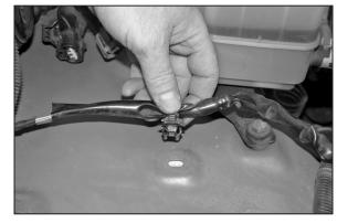
13. Remove the mass air wire harness clip from inner fender.
