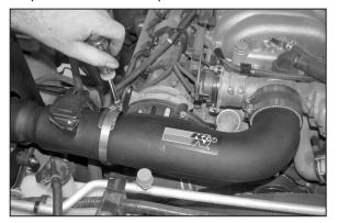
26. Install the K&N® intake tube onto the throttle body and align the tube with the saddle bracket, then tighten all hose clamps to secure intake tube.
