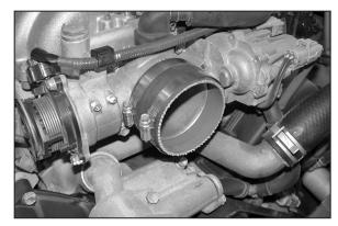
25. Install silicone hose (08690) onto throttle body with provided hose clamps as shown.
