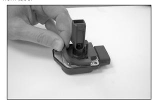
20. Install provided gasket sticky side down as shown.
