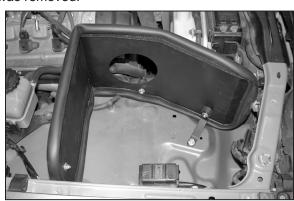
17. Install the heat shield onto vehicle with provided hardware.
