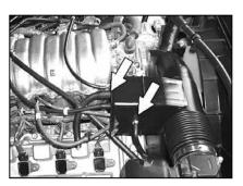
7. Disconnect the four rubber hoses from the engine as shown by the arrows.
