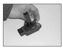
10. Apply the provided gasket to the mass-air sensor with the sticky side down.
