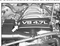
3. Loosen and remove the acorn nuts that secure the throttle body cover, then remove the cover.
