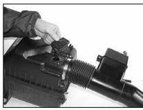
9. Loosen and remove the two screws that secure the mass-air sensor, then remove the mass air sensor.
