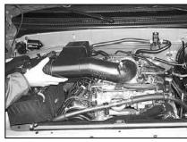
8. Remove the complete air induction system. NOTE: K&N Engineering, Inc., recommends that customers do not discard factory air intake.
