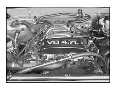
31. Re-install the throttle body cover onto the engine using the original acorn nuts.
