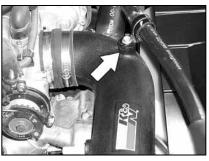
26. Re-connect the AC line to the K&N® intake tube using the original bolt.
