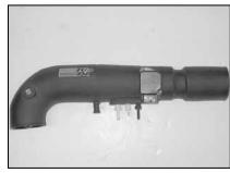
23. On 2000-02 models, install the three vents into the intake tube in the orientation as shown above. NOTE: Plastic NPT fittings are easy to cross thread. Install the vent fitting "hand" tight, then turn it two complete turns with a wrench.
