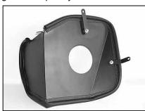
14. Secure the two brackets to the heat shield with the provided hardware, but do not tighten completely.
