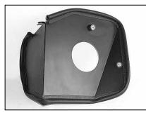
13. Install the two rubber mounted studs to the heat shield with the provided hardware, but do not tighten completely.
