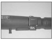
11. Install the mass-air sensor into the K&N® intake tube and secure with the provided spacers and screws as shown.
