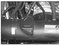
28. Attach the three provided, and one existing hose onto the K&N® intake tube as shown. NOTE: Some '03 models may come equipped with a total of three vacuum lines.
