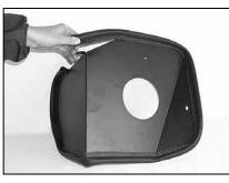
12. Apply the edge trim to the K&N® heat shield as shown above, trim if needed.
