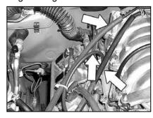
27. Install the three vent hoses onto the engine as shown above. (see arrows)
