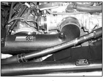
24. Install the K&N® intake tube onto the throttle body and secure with the provided hose clamp.
