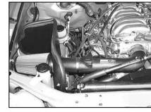
29. Install the K&N® air filter onto the K&N® intake tube as shown.
