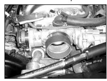
20. Install the silicon hose onto the throttle body and secure it with the provided hose clamp.
